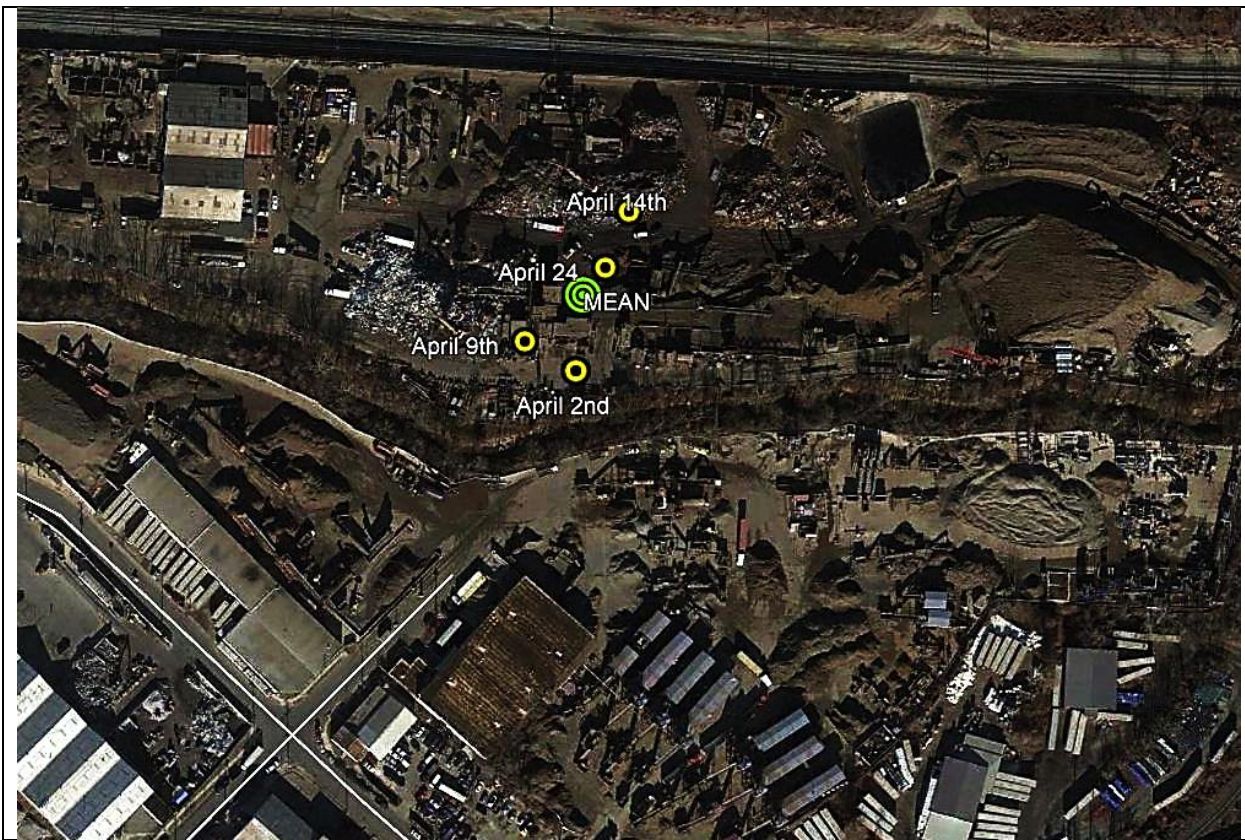
Figure 8.4: The origin of all events plotted as yellow circles with the mean as a green circle. The origin of all events are found to reside within the bounds of Joseph Smith and Son’s – Professional Services Inc. This plot exhibits the precision of location estimations, driven by consistency in time picking methods.
