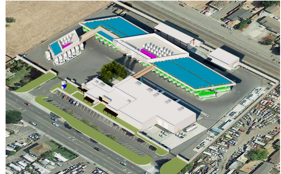
Example – Rendering of Similar Bus Ops Facility with Solar Canopy supporting BEB Charging
